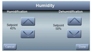
During warm weather periods, under DEHUMIDIFICATION, use the ▲ and ▼ buttons to select your desired humidity level during cooling mode. Press **DONE** to return to normal operation.
