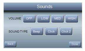
Press **Sounds** from the Basic Setup screen to adjust the Volume and Sound Type heard from your Observer® control. Volume options include: OFF, LOW, MED or HIGH Sound Types include: Beep, Click and Click 2 (Double Click)
