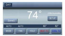
From the **Setup** menu, you can program a comfort schedule for each individual zone by using the  $\blacktriangle/\blacktriangledown$  button to select the corresponding zone.
