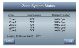
To view the status of each zone, press **Zone Status** to see the current Temperature and Damper Position for each of your installed zones. In addition, the current temperature from the Leaving Air Sensor will also be displayed on this screen.
